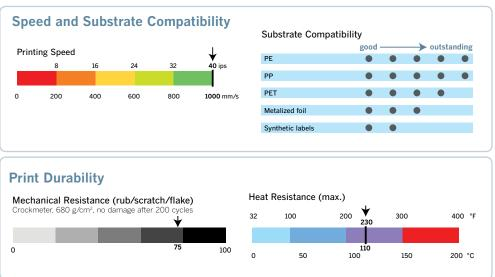
Evaluation of observed performances of the ribbon with optimized printer setting and receptors.
