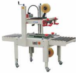
FXJ6050 Carton Sealing Machine 半自动封箱机 Power Supply/供给电压: 110V/220-240V/50-60Hz Power/功率: 180W Conveyor Speed/输送速度: 20m/min Max. Carton Size/最大纸箱尺寸: W500xH600mm Min. Carton Size/最小纸箱尺寸: W150xH120mm Width Of Tape/胶带宽: 50mm or 60mm Machine Size/机器尺寸: 1630x800x1330mm Option: 3inch tape & overlap (Model FXJ6600/3)
