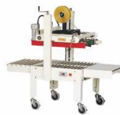
AS123 (Top Sealing Model) Carton Sealing Machine 半自动封箱机 Power Supply/供给电压: 110V/220-240V/50-60Hz Power/功率: 180W Conveyor Speed/输送速度: 20m/min Max. Carton Size/最大纸箱尺寸: W500xH500mm Min. Carton Size/最小纸箱尺寸: W100xH100mm Width Of Tape/胶带宽: 50mm or 60mm Machine Size/机器尺寸: 1545x815x1475mm
