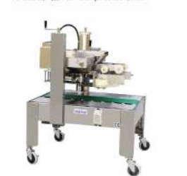
AS623 (Suit for Bubble Box) Carton Side Sealing Machine 半自动封箱机(泡沫箱款) Power Supply/供给电压: 110V/220-240V/50-60Hz Power/功率: 240W Conveyor Speed/输送速度: 20m/min Max. Carton Size/最大纸箱尺寸: W300xH430mm Min. Carton Size/最小纸箱尺寸: W280xH100mm Width Of Tape/胶带宽: 50mm or 60mm
