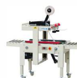
FXJ4030D Carton Side Sealing Machine for E-commerce Box 半自动封箱机(电商款) Power Supply/供给电压: 110V/220-240V/50-60Hz Power/功率: 120W Conveyor Speed/输送速度: 20m/min Max. Carton Size/最大纸箱尺寸: W300xH400mm Min. Carton Size/最小纸箱尺寸: W80xH90mm Width Of Tape/胶带宽: 48mm or 50mm
