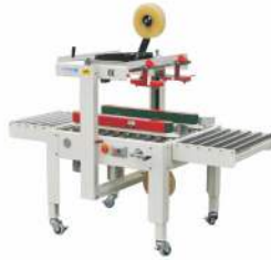
FXJ6600 Carton Sealing Machine 半自动封箱机 Power Supply/供给电压: 110V/220-240V/50-60Hz Power/功率: 180W Conveyor Speed/输送速度: 20m/min Max. Carton Size/最大纸箱尺寸: W500xH600mm Min. Carton Size/最小纸箱尺寸: W100xH100mm Width Of Tape/胶带宽: 50mm or 60mm Machine Size/机器尺寸: 1660x850x1260mm Option: 3inch tape & overlap (Model FXJ6600/3)
