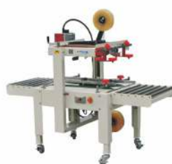
FXJ6600H Carton Sealing Machine 半自动封箱机 Power Supply/供给电压: 110V/220-240V/50-60Hz Power/功率: 180W Conveyor Speed/输送速度: 20m/min Max. Carton Size/最大纸箱尺寸: W500xH600mm Min. Carton Size/最小纸箱尺寸: W100xH100mm Width Of Tape/胶带宽: 50mm or 60mm Machine Size/机器尺寸: 1630x800x1230mm
