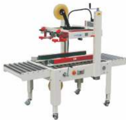
FXJ6050B / FXJ8060B / FXJ9070B Carton Sealing Machine 半自动封箱机 Power Supply/供给电压: 110V/220-240V/50-60Hz Power/功率: 270W Max. Carton Size/最大纸箱尺寸: W500xH600mm(FXJ6050B) Max. Carton Size/最大纸箱尺寸: W600xH800mm(FXJ8060B) Max. Carton Size/最大纸箱尺寸: W700xH900mm(FXJ9070B) Min. Carton Size/最小纸箱尺寸: W150xH120mm Width Of Tape/胶带宽: 50mm or 60mm or 75mm
