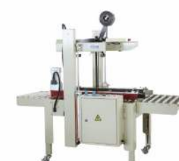
AS823A (Random Model) Carton Sealing Machine for Random size box 半自动封箱机(自动尺寸调节款) Power Supply/供给电压: 110V/220-240V/50-60Hz Power/功率: 240W Conveyor Speed/输送速度: 20m/min Max. Carton Size/最大纸箱尺寸: W500xH500mm Min. Carton Size/最小纸箱尺寸: W150xH120mm Width Of Tape/胶带宽: 50mm or 60mm Air Source/气源: 0.4-0.8Mpa @ 450l/min.
