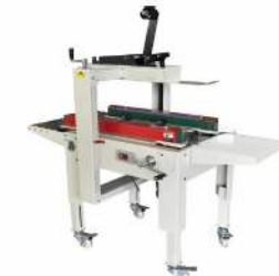
FXJ4030X Carton Side Sealing Machine for E-commerce Box 半自动封箱机(电商款) Power Supply/供给电压: 110V/220-240V/50-60Hz Power/功率: 120W Conveyor Speed/输送速度: 20m/min Max. Carton Size/最大纸箱尺寸: W300xH400mm Min. Carton Size/最小纸箱尺寸: W80xH90mm Width Of Tape/胶带宽: 48mm or 50mm
