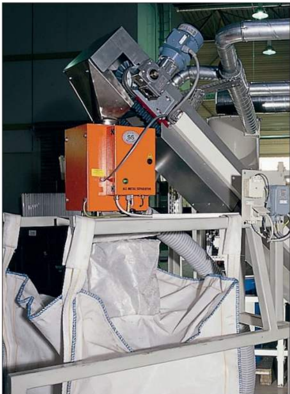
Metal separator RAPID COMPACT used for the quality control of plastic granulate
