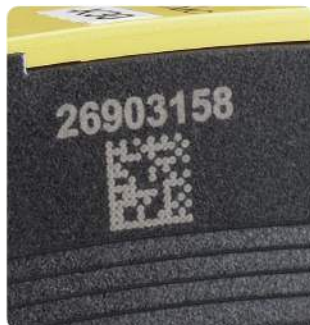
UV laser code on plastic
