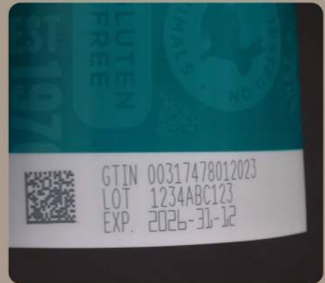
UV laser code on flexible film
